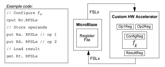
Figure 1-12: FSL used with HW accelerated function  $f_X$
